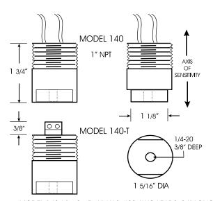
MODEL 140 (-1, -2, -5, -X) HAS #20 AWG LEADS, 24" LONG MODEL 140-T (-1, -2, -5, -X) HAS TERMINAL STRIP
